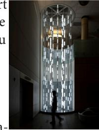
Snow Words is a light sculpture in Alaska inspired by Balmond's template of primes. LED acrylic lights are gapped on stainless steel bar and stainless steel plates. It is 9m high, about 2.7m wide. There are two rings, one within the other. A computer controls the LED lights to create a growing, swelling, diminishing around in two circles. It won a national award in America.
